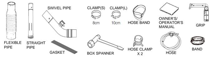
STEP #2) Attach the gasket to the SWIVEL PIPE. Peel off the gasket paper and attach it to the SWIVEL PIPE as shown in the figure.
