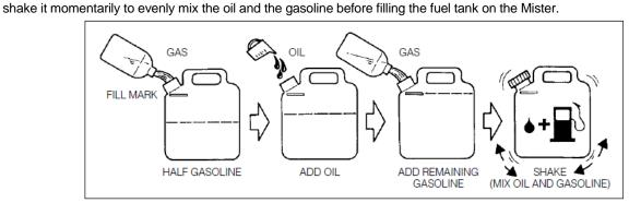
When refilling the Mister fuel tank, clean around the fuel tank cap to prevent dirt and debris for entering the tank during cap removal. Always shake the premix fuel container momentarily before filling the fuel tank.
