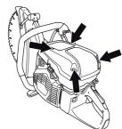
• Check the air filter and replace if necessary.
