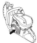
NOTICE! A dirty or blocked air intake results in the machine overheating which causes damage to the piston and cylinder.
