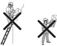
• Always hold the machine in a firm grip with both hands. Hold it so that the thumbs and fingers grip round the handles.
