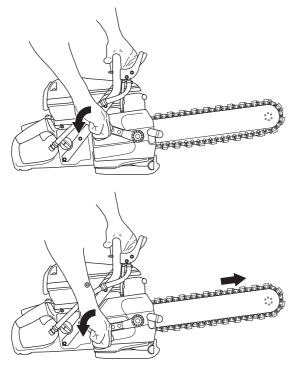
· Hold the bar upwards as you move the handle forward.
