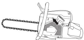
**Stop switch:** Make sure that the stop switch (STOP) is in the left position.
