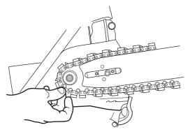
• Remove the spring holding the two "half-moons" using a screwdriver.
