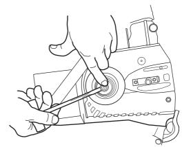
• Remove the "halfmoons", the cup guard, o-ring and the drive sprocket.
