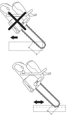
In principle there are two ways to start the process of entering a thick object to be cut.
