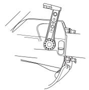
• Move the lever to its rear, lower position. Push in the spring on the chain tensioner handle and turn the bar nut clockwise by hand.
