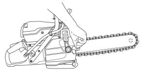
A correctly tightened chain should be easy to pull around by hand.
