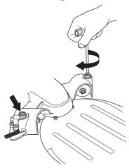
Adjust so you can easily stop the support rollers using your thumb when the blade is rotated. The support rollers should only follow the blade occasionally.
