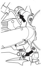
Pump in grease until clean grease emerges from the overflow hole.
