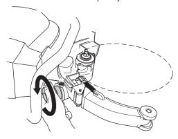
The guide roller can now be pulled out of the chassis.
