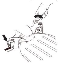
Unscrew the adjuster screws a few turns.
