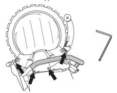
Use a 19 mm fixed spanner and a 13 mm combination spanner to replace the rollers.
