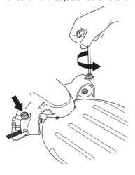
· Loosen the knob to offload the springs.
