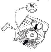
Remove the recoil spring by turning the starter over and loosen the hooks, with the help of a screwdriver. The hooks hold the return spring assembly on the starter.
