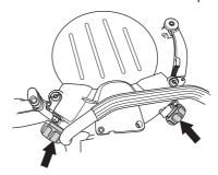
Remove the four screws holding the support roller guard using a 6 mm hex key and lift off the cover.
