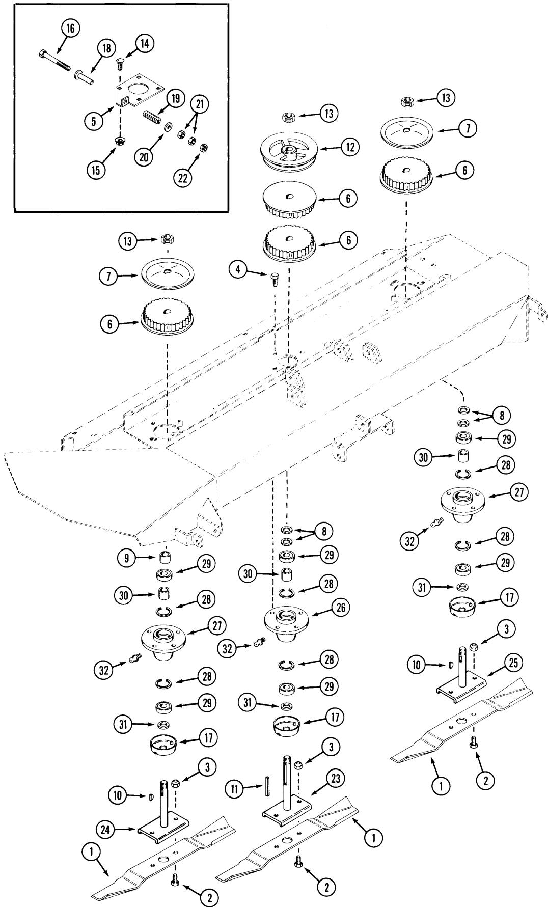
**INDEX****AHRM60 ROTARY MOWER****PULLEYS, BLADES AND SPINDLES**
